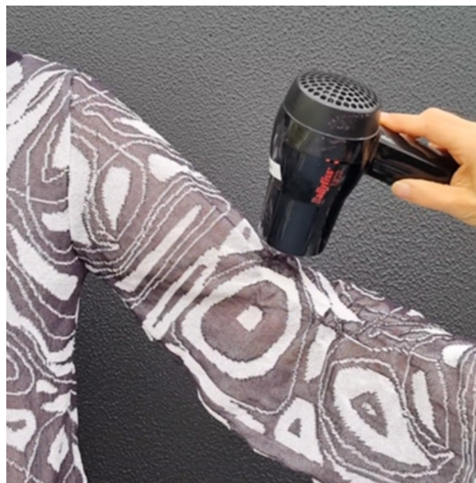
Fig 1. In this sample, only the white yarn reacts to heat by contracting. This creates an uneven surface texture and changes the fit of the garment.
