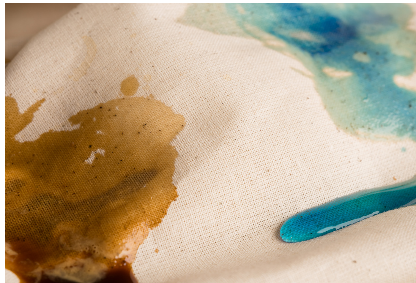
Figure 3. Cotton fabric stained with coffee and Methylene Blue (MB) dyes. These dyes were used to evaluate the self-cleaning properties of ZnO-coated samples. Author: Mikael Nyberg, UTU.
