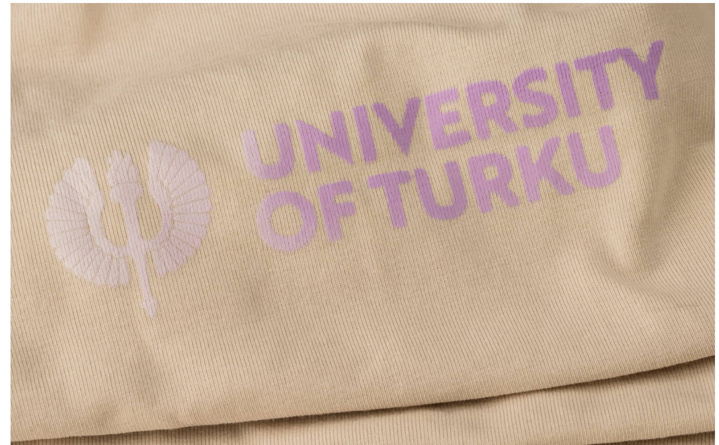
Figure 3. Hackmanite-loaded coating applied on an ordinary cotton T-shirt. Partial coloration changes under UV light. Author: Mikael Nyberg, UTU.
